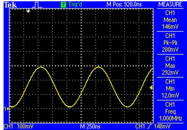
Figure 3. DDS Output When Amplitude Control DAC Is Set to 0.6 V (This Produces One-Half Scale DDS Output)
