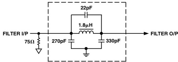
Figure 92. Output Filter Used with Output Buffer
