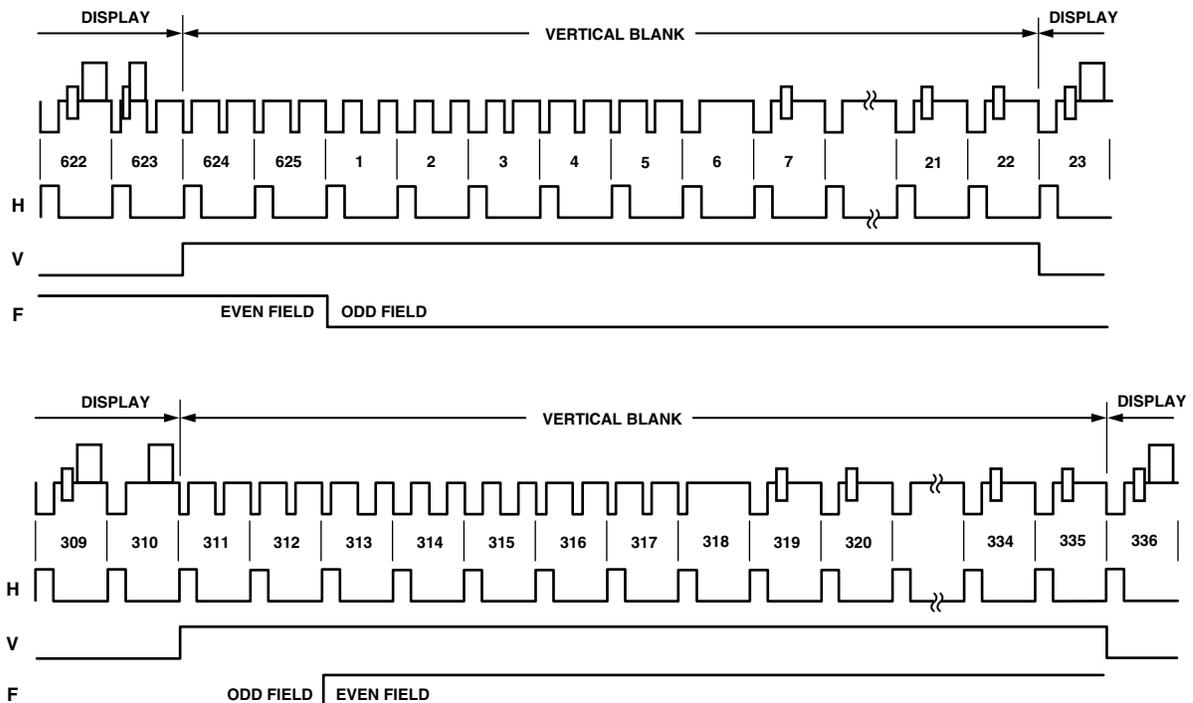
Figure 25. Timing Mode 0 (PAL Master Mode)
