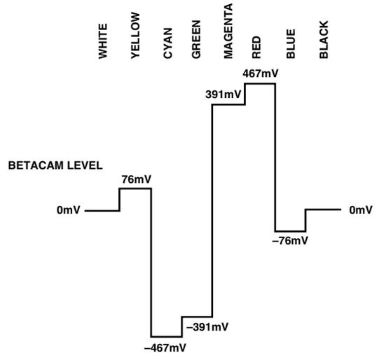
Figure 90. NTSC 100% Color Bars with Pedestal V Levels
