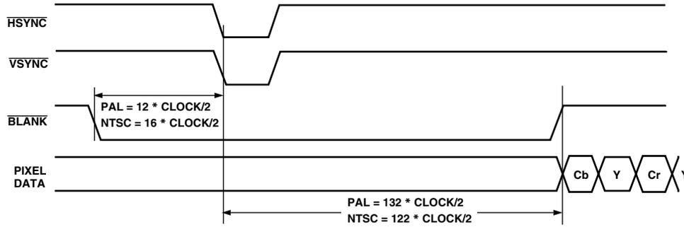
Figure 32. Timing Mode 2 Even-to-Odd Field Transition Master/Slave
