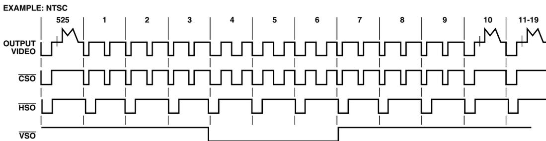
Figure 37.  $\overline{CSO}$ ,  $\overline{HSO}$ ,  $\overline{VSO}$  Timing Diagram
