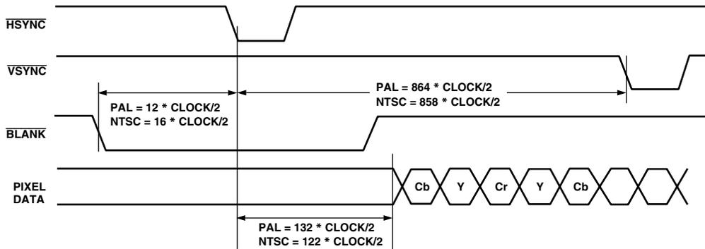
Figure 33. Timing Mode 2 Odd-to-Even Field Transition Master/Slave
