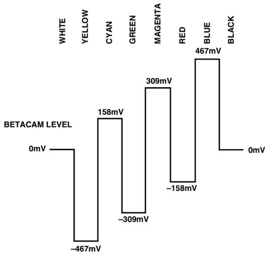
Figure 87. NTSC 100% Color Bars with Pedestal U Levels
