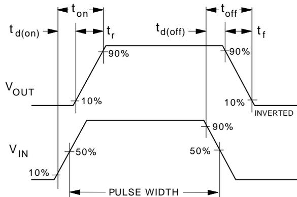
Figure 12. Switching Waveforms.
