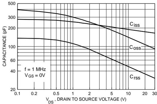
Figure 9. Capacitance Characteristics.
