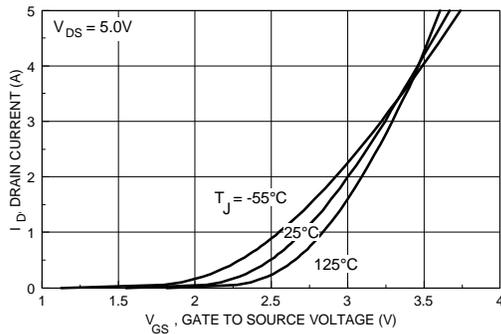
Figure 5. Transfer Characteristics.
