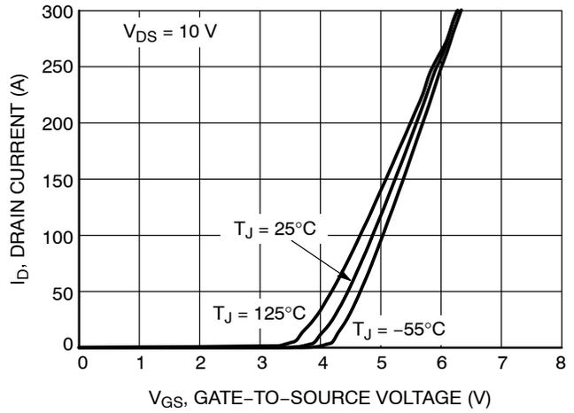
Figure 2. Transfer Characteristics
