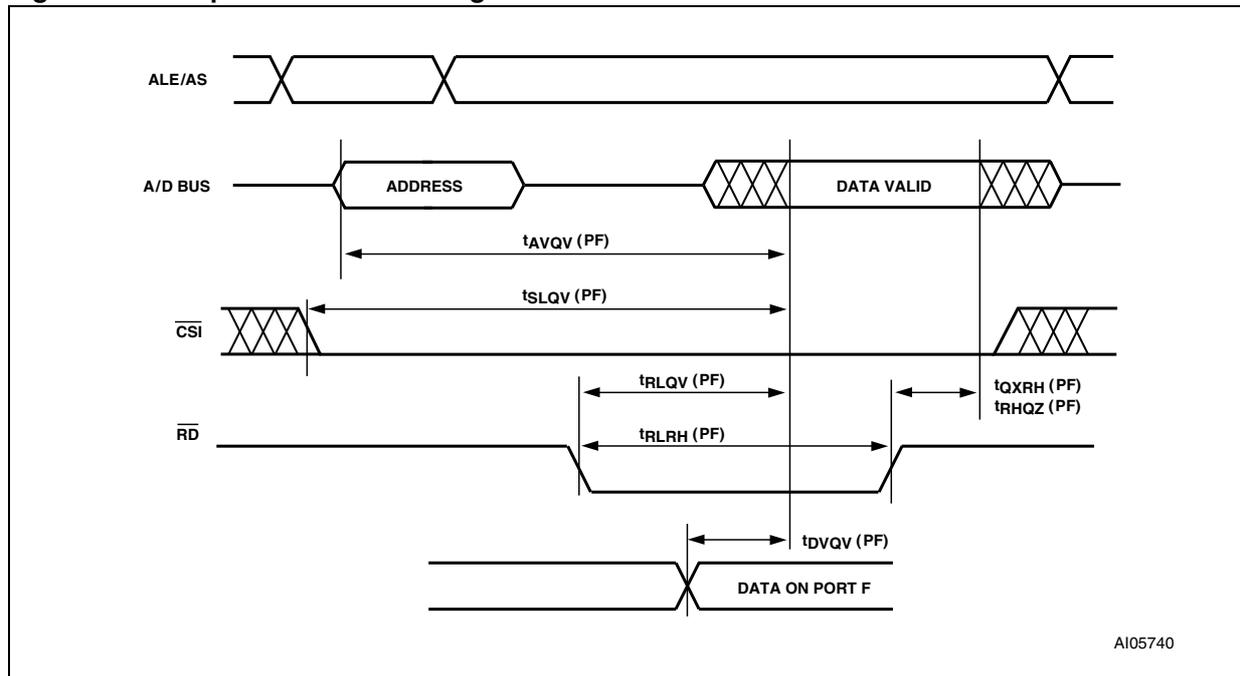
**Table 69. Port F Peripheral Data Mode Read timing**
