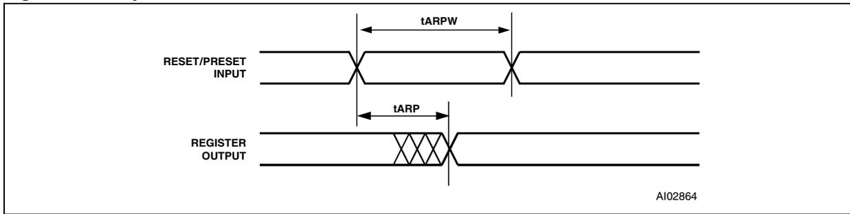
Figure 41. Asynchronous clock mode timing (product term clock)
