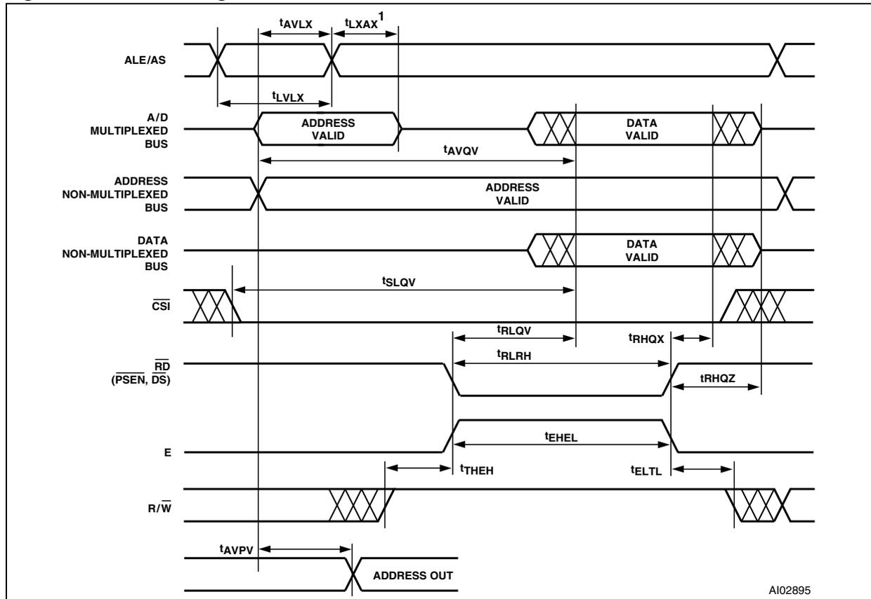
1.  $t_{AVLX}$  and  $t_{LXAX}$  are not required for 80C251 in Page Mode or 80C51XA in Burst Mode.
