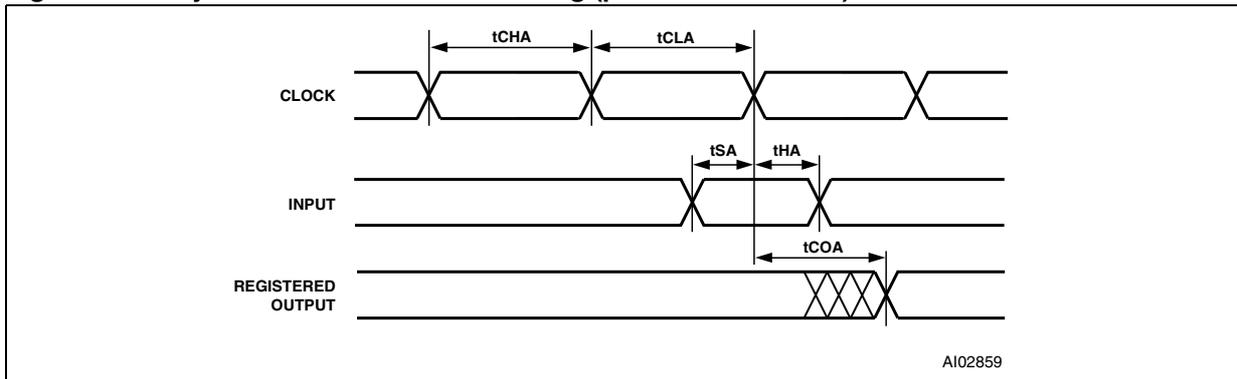
Figure 42. Input macrocell timing (product term clock)
