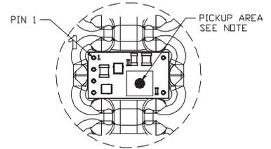
NOTE: THE INDUCTOR IS USED TO PICK AND PLACE THE MODULE. IT'S LOCATION MAY VARY FROM PACKAGE STYLE, SEE PRODUCT TABLE
