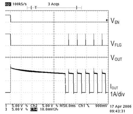
Fig. 19: Short Circuit Response (Enable to Short Circuit)
