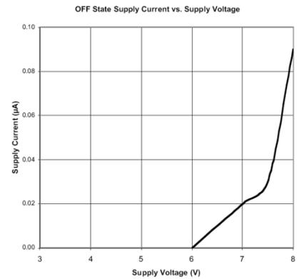
Fig. 9: Off-state Supply Current vs Supply Voltage
