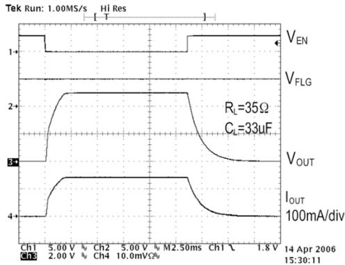
Fig. 16: Turn-On, Turn-Off Characteristics
