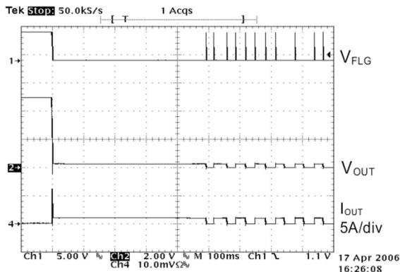
Fig. 18: Short Circuit Response (Short applied to Output)
