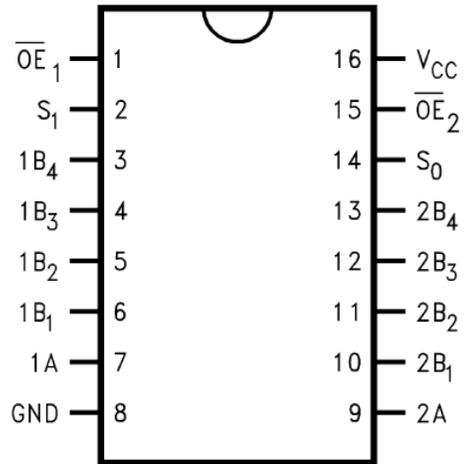
Figure 2. Pin Assignments
