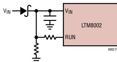
**Figure 4. The Input Diode Prevents a Shorted Input from Discharging a Backup Battery Tied to the Output. It Also Protects the Circuit from a Reversed Input. The LTM8002 Runs Only When the Input Is Present**
