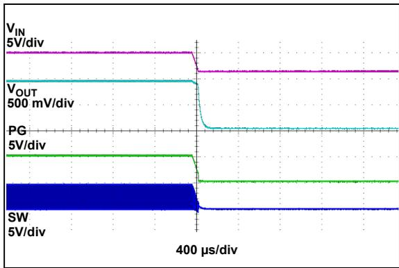
FIGURE 2-20:  $V_{IN}$  Turn-Off ( $EN = PV_{IN}$ ),  $R_{LOAD} = 0.3\Omega$ .
