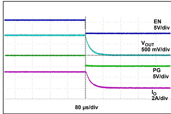
FIGURE 2-22:  $EN$  Turn-Off,  $R_{LOAD} = 0.3\Omega$ .
