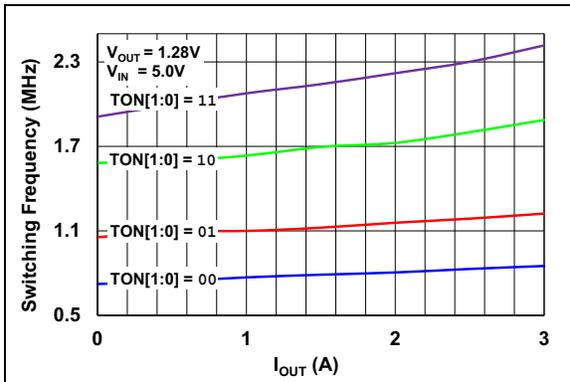
**FIGURE 2-15:** Switching Frequency vs.  $I_{OUT}$  ( $V_{OUT} = 1.28V$ ).
