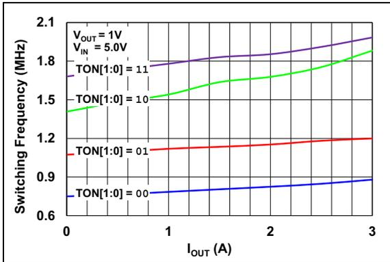
**FIGURE 2-14:** Switching Frequency vs.  $I_{OUT}$  ( $V_{OUT} = 1.0V$ ).
