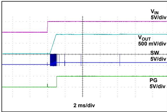
FIGURE 2-19:  $V_{IN}$  Turn-On ( $EN = PV_{IN}$ ).
