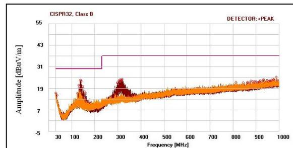
**FIGURE 1:** Radiated Emissions, CISPR32, Class B ( $V_{IN} = 5V$ ,  $V_{OUT} = 1V$ ,  $I_{OUT} = 3A$ ).
