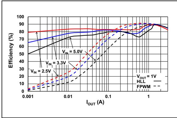
**FIGURE 2-7:** Efficiency vs. Load Current ( $V_{OUT} = 1.0V$ ).
