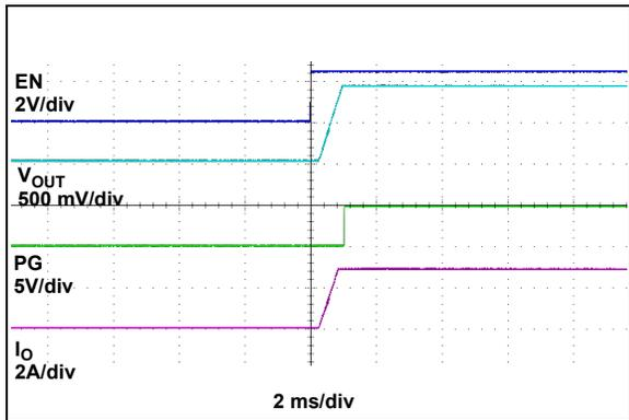
FIGURE 2-21:  $EN$  Turn-On,  $R_{LOAD} = 0.3\Omega$ .
