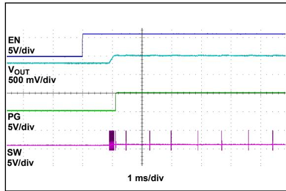
FIGURE 2-23:  $EN$  Turn-On into Pre-Biased Output ( $V_{pre-bias} = 0.8V$ ).
