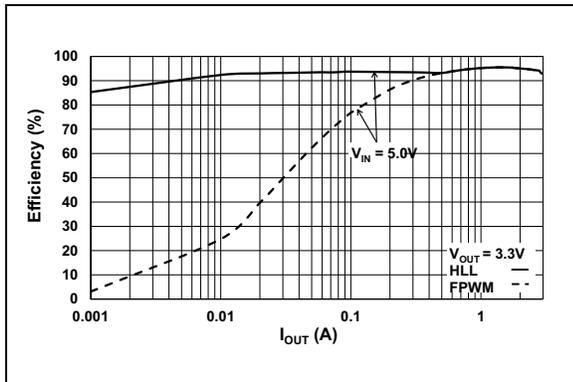
**FIGURE 2-9:** Efficiency vs. Load Current ( $V_{OUT} = 3.3V$ ).
