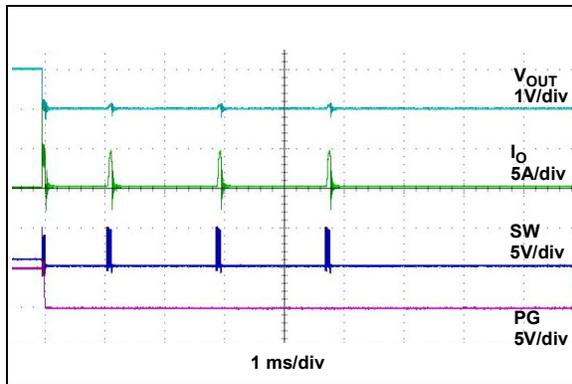
**FIGURE 2-26:** Hiccup Mode Short-Circuit Current Limit Response.
