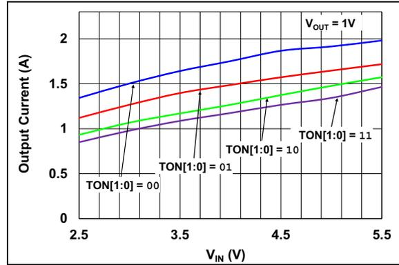
**FIGURE 2-10:** DCM/FPWM  $I_{OUT}$  Threshold vs.  $V_{IN}$ .
