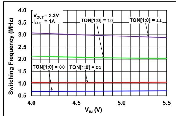
**FIGURE 2-18:** Switching Frequency vs.  $V_{IN}$  ( $V_{OUT} = 3.3V$ ).
