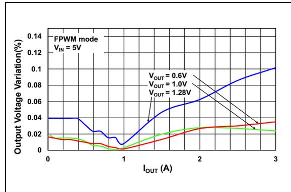
**FIGURE 2-12:** Load Regulation: Output Voltage Variation vs.  $I_{OUT}$ .
