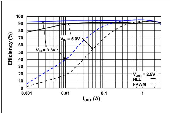
**FIGURE 2-8:** Efficiency vs. Load Current ( $V_{OUT} = 2.5V$ ).
