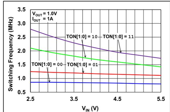
**FIGURE 2-17:** Switching Frequency vs.  $V_{IN}$  ( $V_{OUT} = 1.0V$ ).
