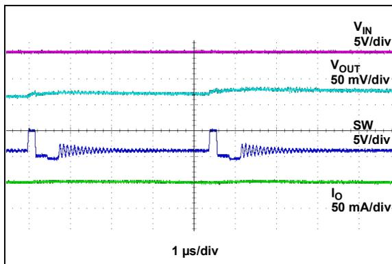
**FIGURE 2-27:** Switching Waveforms –  $I_{OUT} = 50 \text{ mA}$ , HLL.
