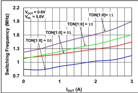
**FIGURE 2-13:** Switching Frequency vs.  $I_{OUT}$  ( $V_{OUT} = 0.6V$ ).
