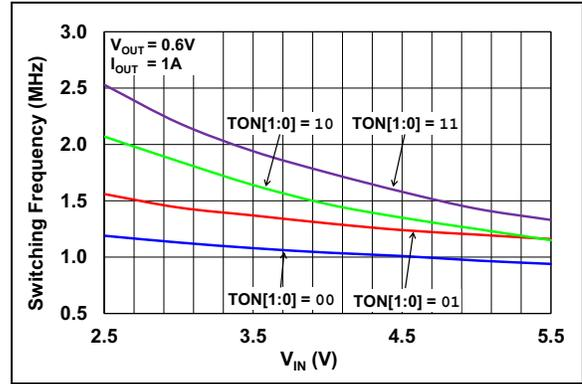
**FIGURE 2-16:** Switching Frequency vs.  $V_{IN}$  ( $V_{OUT} = 0.6V$ ).
