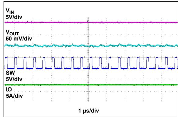
**FIGURE 2-28:** Switching Waveforms –  $I_{OUT} = 3A$ .
