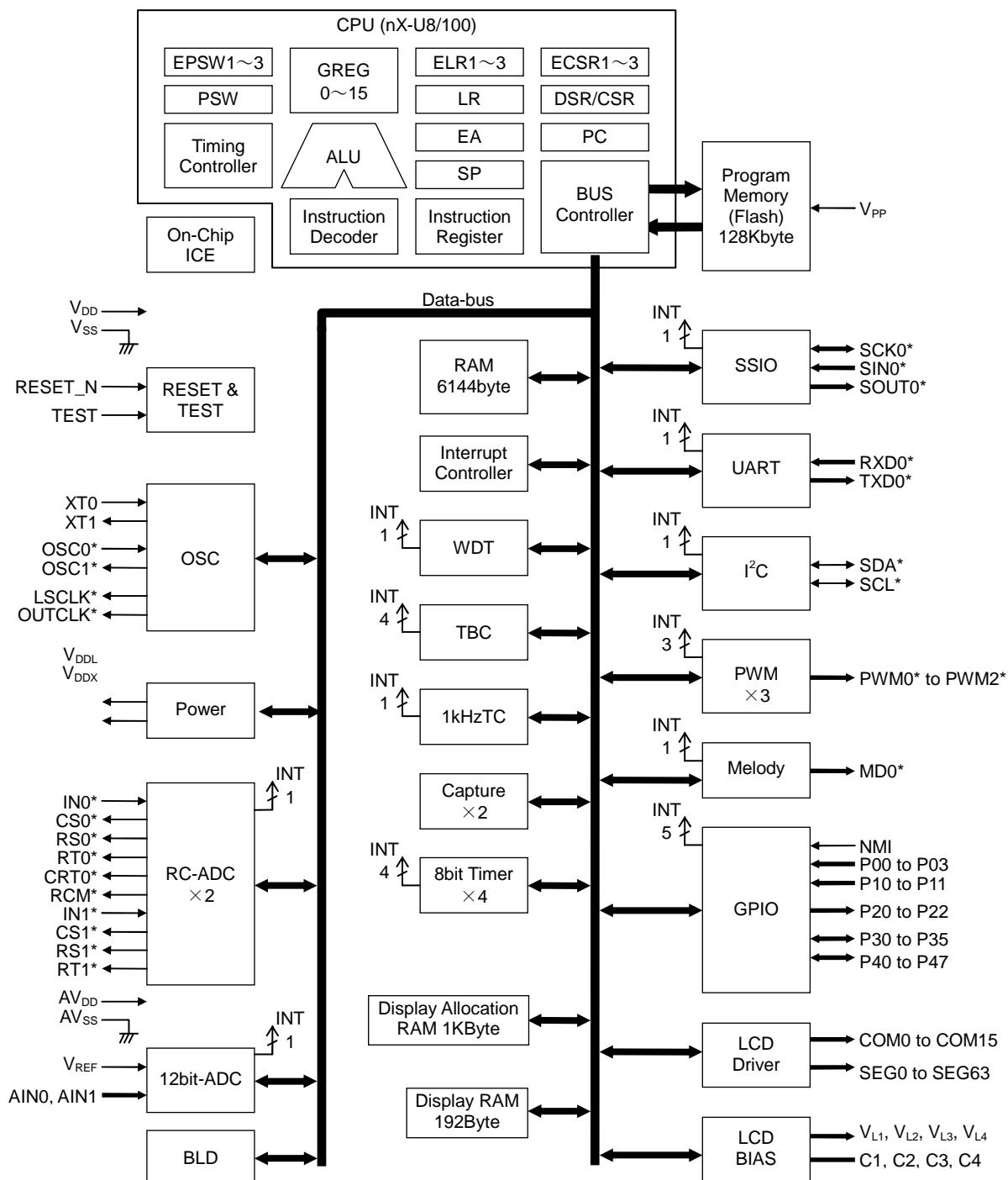
Figure 2 ML610Q439 Block Diagram
