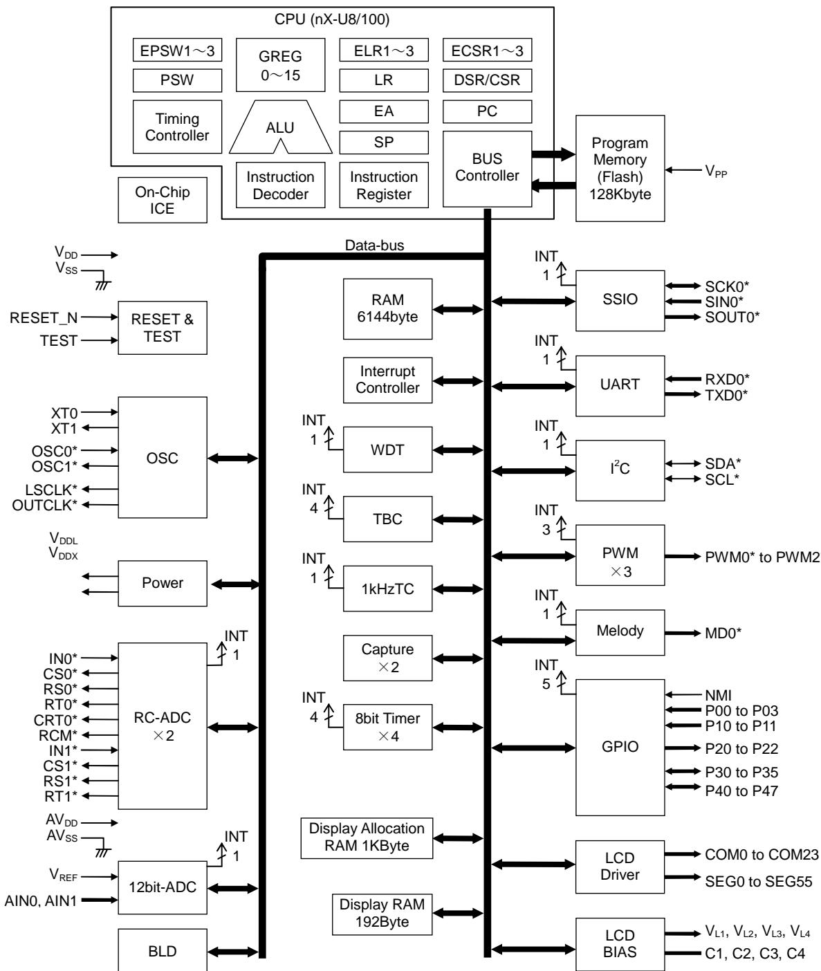
**Figure 1 ML610Q438 Block Diagram**
