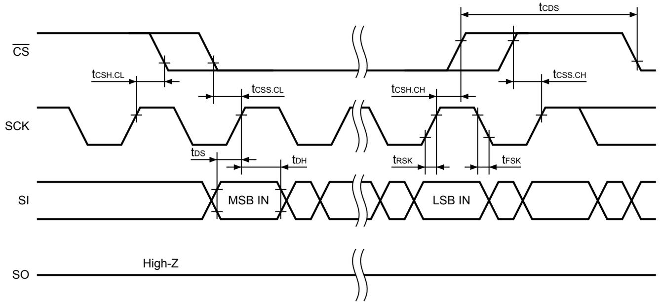
Figure 5 Serial Input Timing
