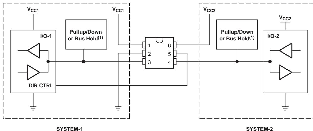
The following table shows data transmission from SYSTEM-1 to SYSTEM-2 and then from SYSTEM-2 to SYSTEM-1.
