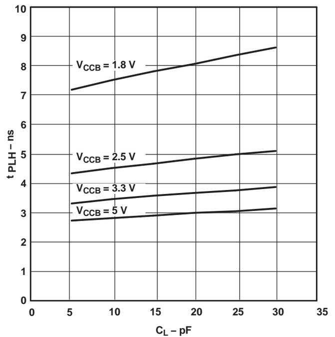
**TYPICAL PROPAGATION DELAY (B to A) vs LOAD CAPACITANCE**
