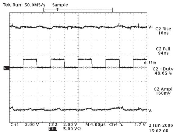
SP3244 Charge Pump Waveforms for 250kbps
