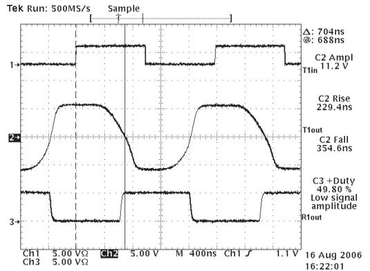
SP2345 Waveforms for 1Mbps Clock Rate
