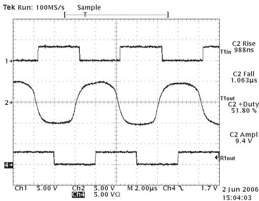
SP3244 Waveforms for 250kbps Clock Rate
