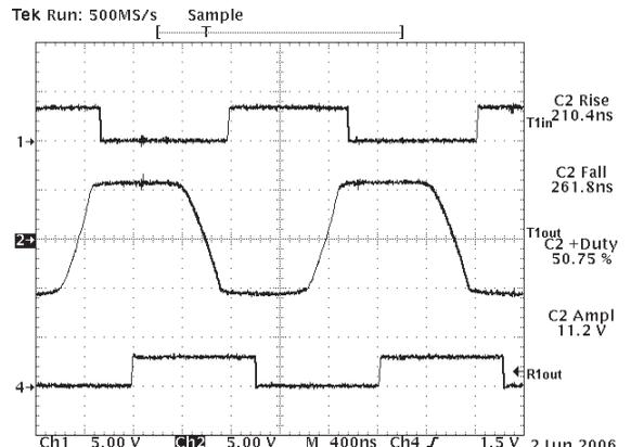
SP3244 Waveforms for 1Mbps Clock Rate
