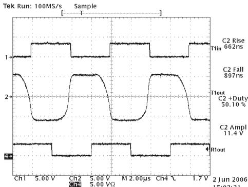
SP3244 Waveforms for 250kbps Clock Rate
