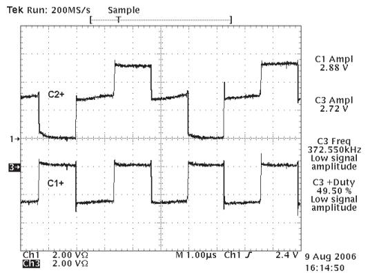
SP3244 C2+ Charge Pump Waveforms - Vcc=3.3V,
