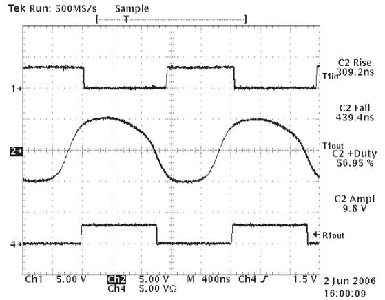
SP3244 Waveforms for 1Mbps Clock Rate
