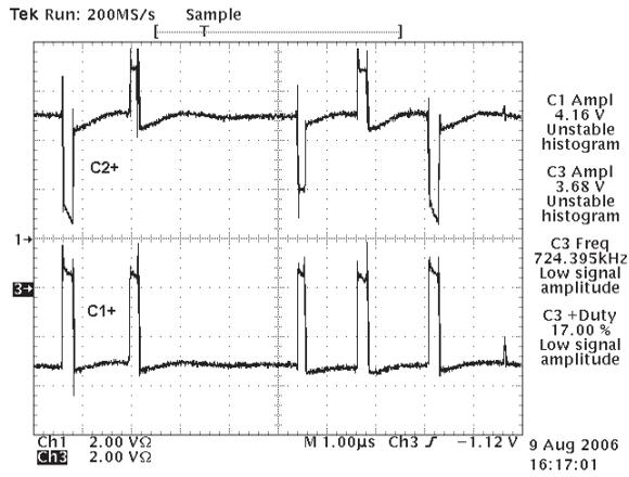
SP3244 C2+ Charge Pump Waveforms -
