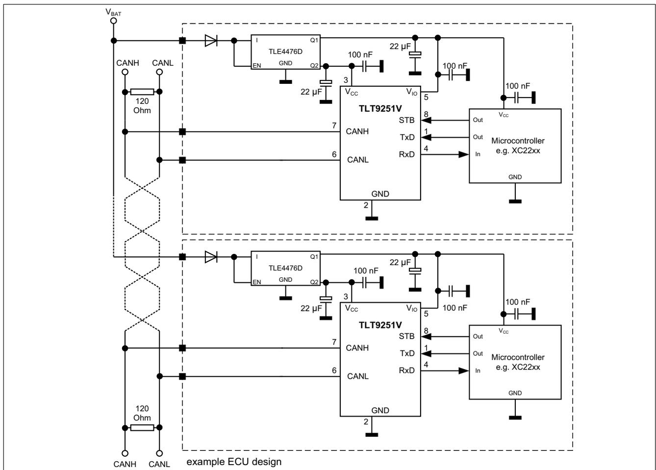
**Figure 18 Application circuit**
