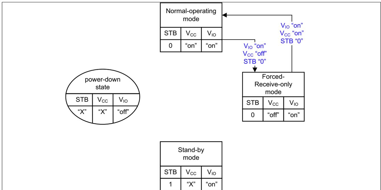
Figure 8 Mode changes by undervoltage events on  $V_{CC}$
