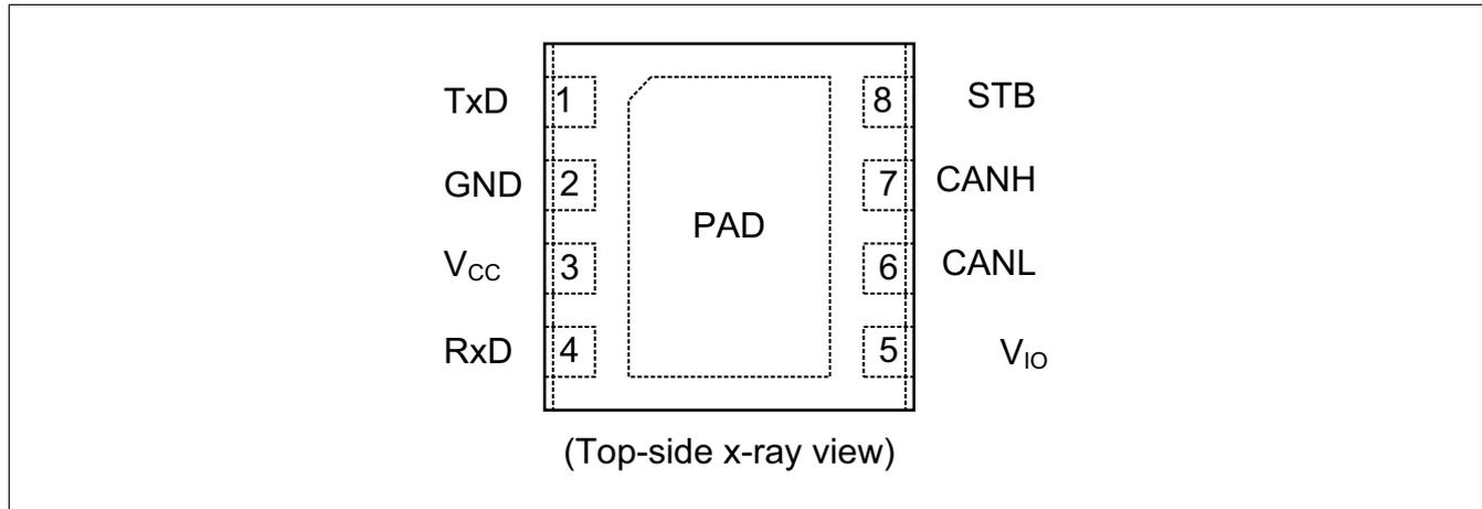
Figure 2 Pin configuration
