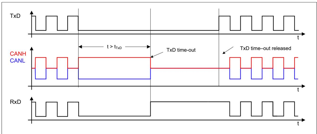
Figure 13 TxD time-out function
