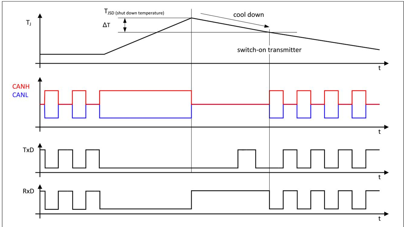
**Figure 14 Overtemperature protection**
