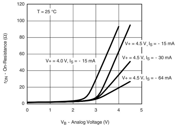
**r<sub>ON</sub> vs. V<sub>B</sub> Single Supply Voltage**
