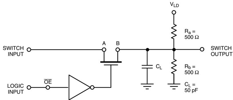
Input driven by  $50 \Omega$  source terminated in  $50 \Omega$
