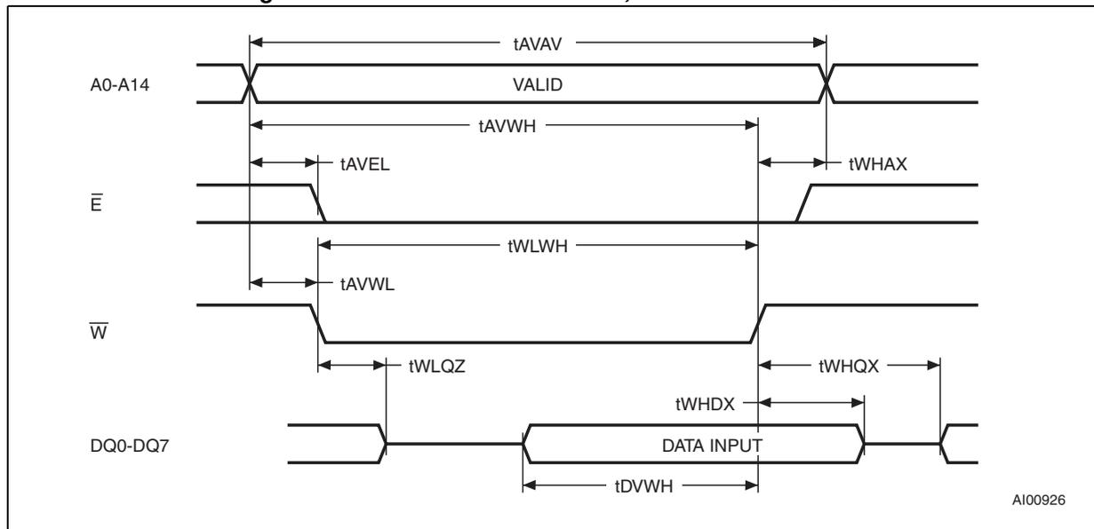
Figure 7. Chip enable controlled, WRITE AC waveforms
