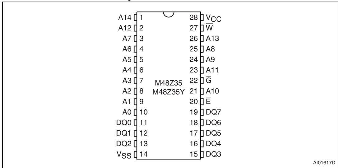
Figure 3. SOIC connections
