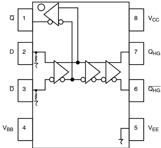
**Figure 1. 8-Lead Pinout (Top View) and Logic Diagram**
