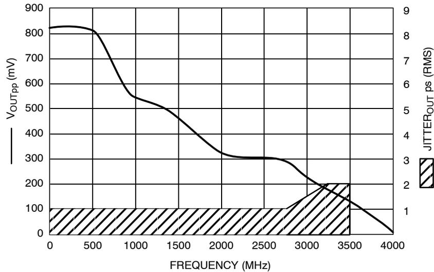
Figure 3. F<sub>max</sub>/Jitter for Q̄ Output
