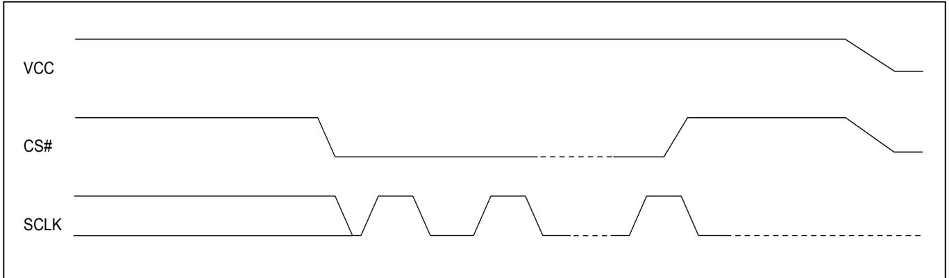
**Figure 34. Power-up Timing**
