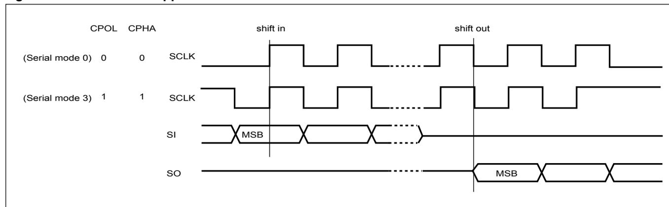
**Note:** CPOL indicates clock polarity of Serial master:
