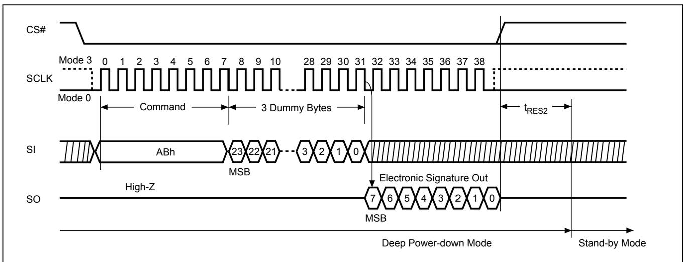
**Figure 25. Release from Deep Power-down (RDP) Sequence**
