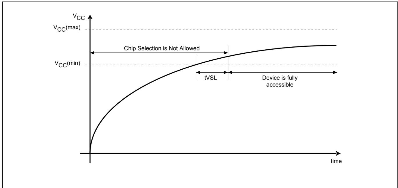
**Figure 35. Power Up/Down and Voltage Drop**
