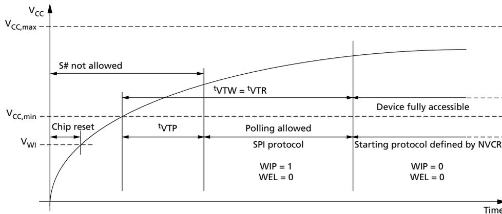
**Table 35: Power-Up Timing and  $V_{WI}$  Threshold**
