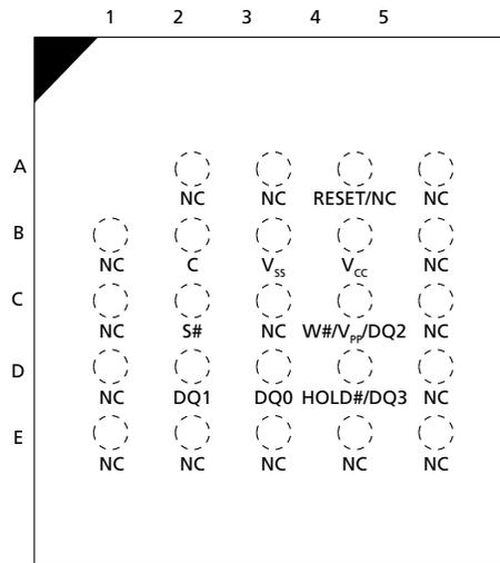
Note: 1. See Part Number Ordering Information for complete package names and details. Ball A4 is NC except for part numbers N25Q512A83G1240x, N25Q512A83G12A0x and N25Q512A83G12H0x for which it is used as a RESET pin.
