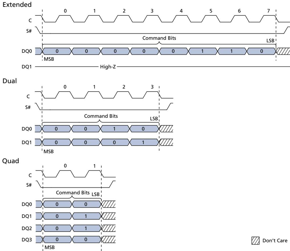
Note: 1. Shown here is the WRITE ENABLE command code, which is 06h or 0000 0110 binary. The WRITE DISABLE command sequence is identical, except the WRITE DISABLE command code is 04h or 0000 0100 binary.
