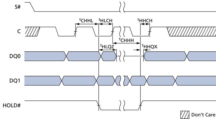
**Figure 44: Output Timing**
