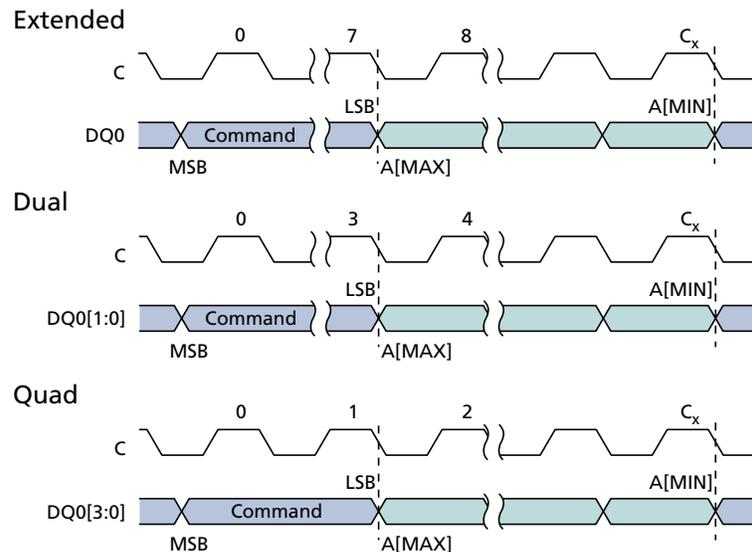
Note: 1. For extended SPI protocol,  $C_x = 7 + (A[\text{MAX}] + 1)$ .
