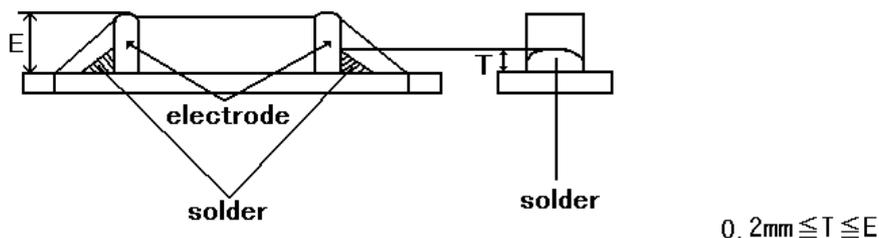
iii. Too much solder gives too strong mechanical stress to this product, such stress may cause cracking or any mechanical damage. And also, it can destroy the electrical performance of this product.
