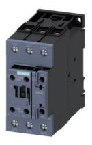
power contactor, AC-3 51 A, 22 kW / 400 V 1 NO + 1 NC, 24 V DC with varistor, 3-pole, size S2, screw terminal upright mounting position suitable for 2 A PLC outputs
