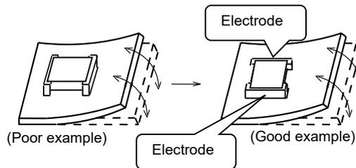
(2) Components location on PCB separation
