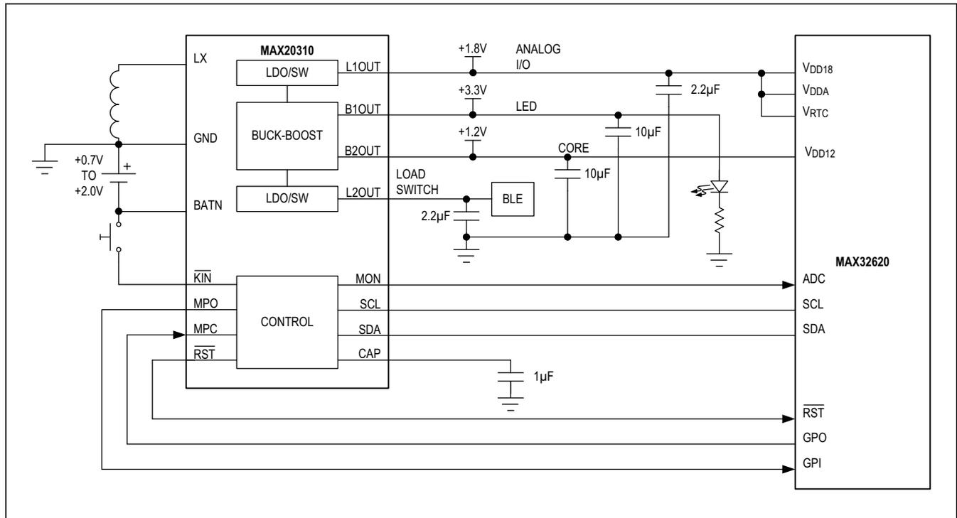
**Note:** The capacitor values shown reflect an effective capacitance. Derate capacitors appropriately according to specific application requirements.
