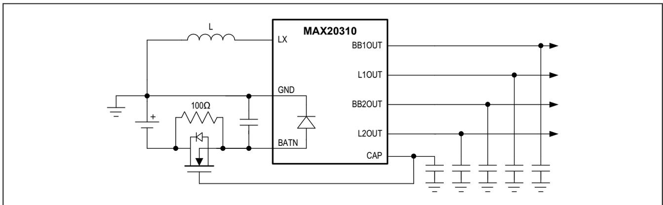
Figure 2. Reverse Battery Protection Using an External MOSFET
