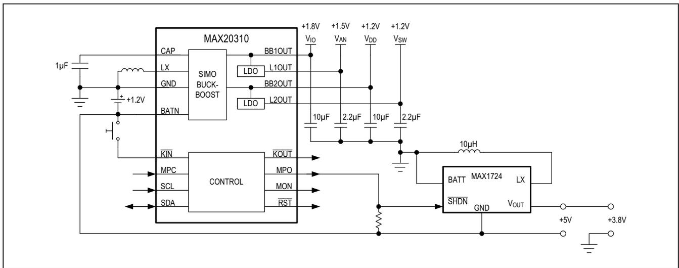
Figure 1. Controlling an External Regulator with MPO
