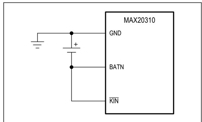
Figure 4.  $\overline{\text{KIN}}$  Connected to BATN for Always-On Applications
