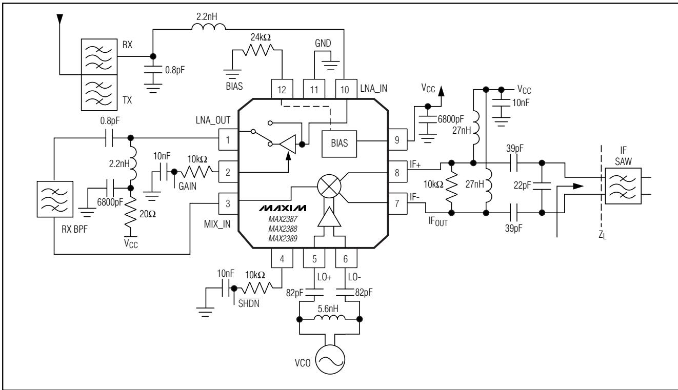
Figure 2. MAX2387/MAX2388/MAX2389 Differential IF Load; Differential VCO
