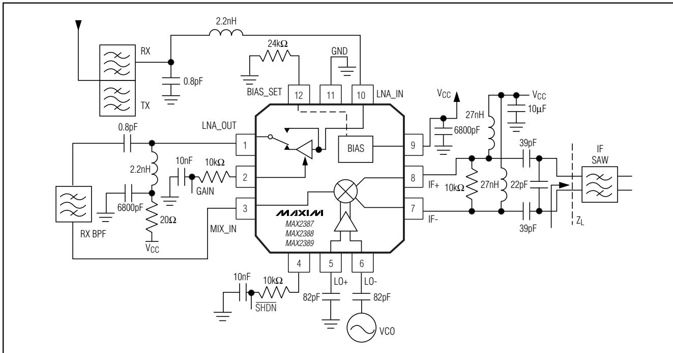
Figure 1. MAX2387/MAX2388/MAX2389 Differential IF Load; Single-Ended VCO
