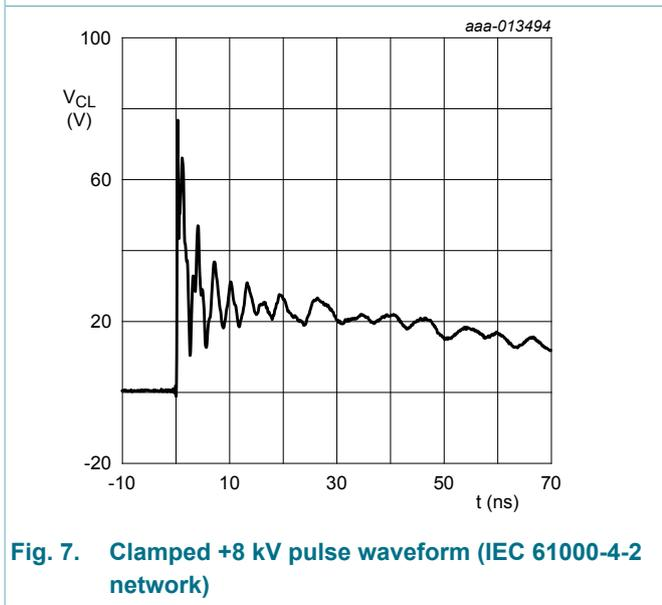
Fig. 7. Clamped +8 kV pulse waveform (IEC 61000-4-2 network)
