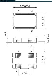
PAD FUNCTION: 1:ENABLE CONTROL 2:GND 3:OUT 4:VDD
