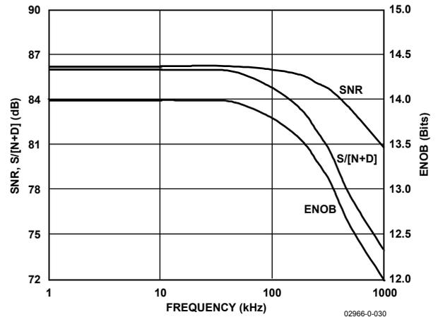
Figure 10. SNR, S/(N+D), and ENOB vs. Frequency
