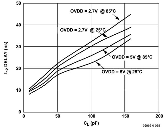
Figure 19. Typical Delay vs. Load Capacitance  $C_L$
