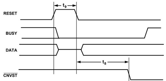
Figure 27. RESET Timing
