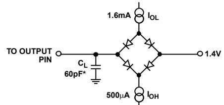
\*IN SERIAL INTERFACE MODES, THE SYNC, SCLK, AND SDO<sub>UT</sub> TIMINGS ARE DEFINED WITH A MAXIMUM LOAD  $C_L$  OF 10pF; OTHERWISE, THE LOAD IS 60pF MAXIMUM.
