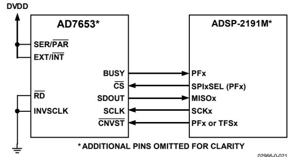
Figure 37. Interfacing the AD7653 to an SPI Interface
