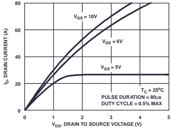
**Figure 8. Saturation Characteristics**
