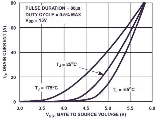
**Figure 7. Transfer Characteristics**
