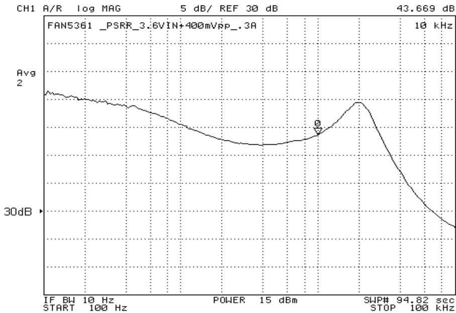
Figure 40. Power Supply Rejection Ratio at 300 mA Load
