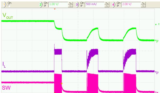
**Figure 35. Over-Current Fault Response,  $R_{LOAD} = 1\ \Omega$ ,  $50\ \mu\text{s}/\text{div}$ .**
