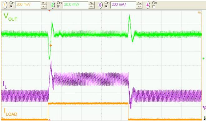
Figure 26. Load Transient 150 to 400 mA, 2.5  $V_{IN}$
