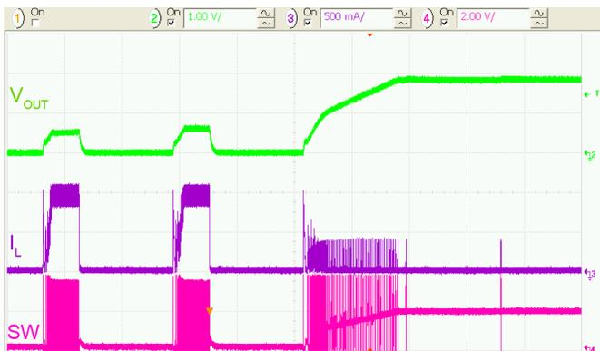
**Figure 37. Overload Recovery to Light Load,  $50\ \mu\text{s}/\text{div}$ .**
