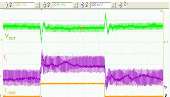
Figure 29. Load Transient 150 to 400 mA, 3.6  $V_{IN}$
