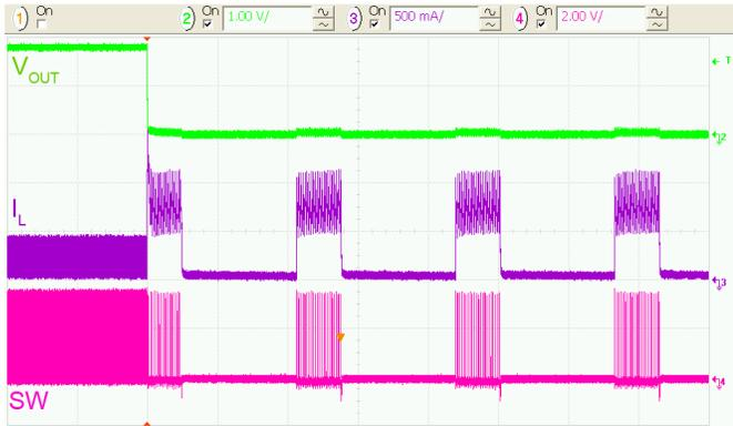
**Figure 33. Metallic Short Applied at  $V_{OUT}$ ,  $50\ \mu\text{s}/\text{div}$ .**
