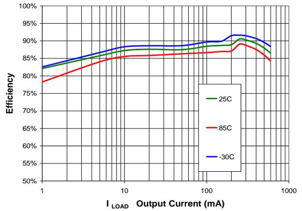
Figure 6. Efficiency vs. Load Current and Temperature
