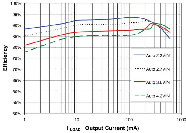
Figure 5. Efficiency vs. Load Current and Input Supply
