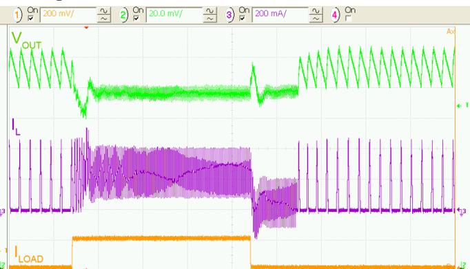
Figure 31. Load Transient 50 to 250 mA, 4.5  $V_{IN}$
