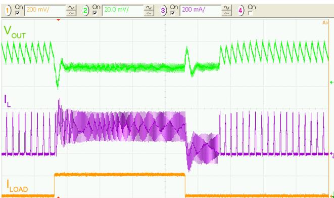
Figure 28. Load Transient 50 to 250 mA, 3.6  $V_{IN}$
