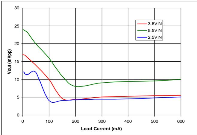
**Figure 13. 1.233 V<sub>OUT</sub> Peak-to-Peak Output Voltage Ripple**
