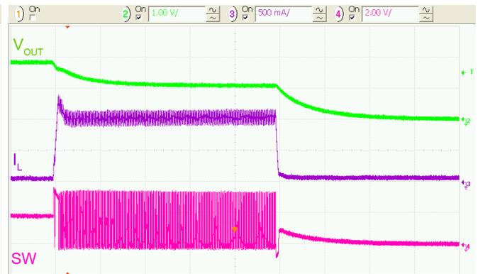
**Figure 36. Over-Current Fault Response,  $R_{LOAD} = 1\ \Omega$**
