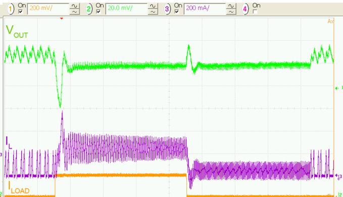
**Figure 25.** Load Transient 50 to 250 mA, 2.5  $V_{IN}$
