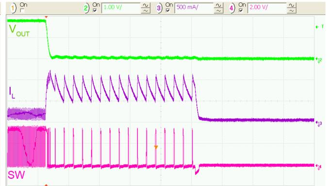
**Figure 34. Metallic Short Applied at  $V_{OUT}$**
