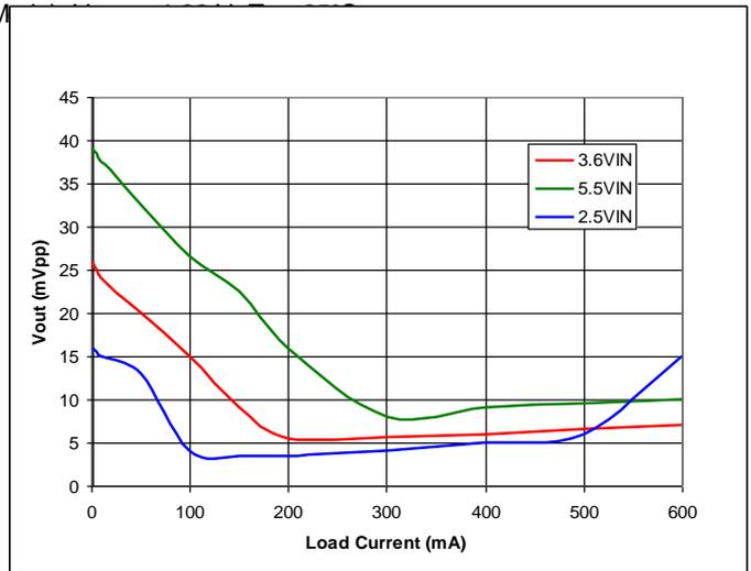
**Figure 12. 1.82 V<sub>OUT</sub> Peak-to-Peak Output Voltage Ripple**
