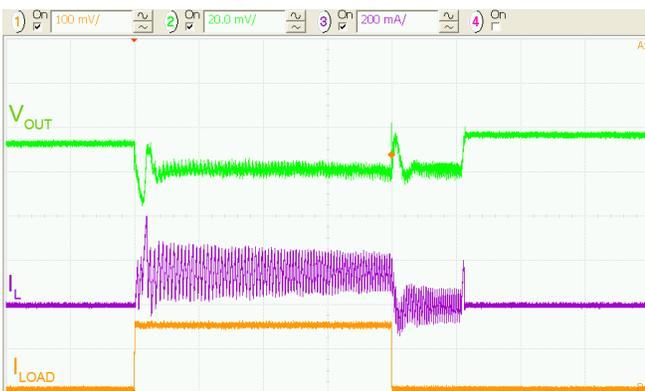
**Figure 24.** Load Transient 0 to 150 mA, 2.5  $V_{IN}$
