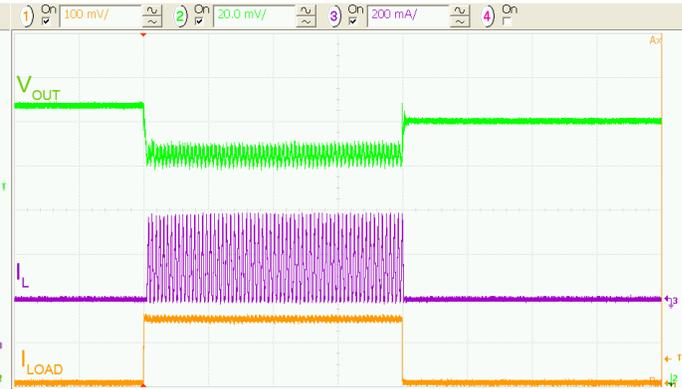
Figure 27. Load Transient 0 to 150 mA, 3.6  $V_{IN}$
