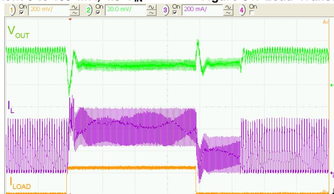
Figure 32. Load Transient 150 to 400 mA, 4.5  $V_{IN}$
