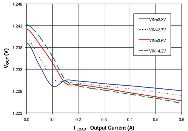
Figure 10. 1.233  $V_{OUT}$  Load Regulation vs. Input Supply
