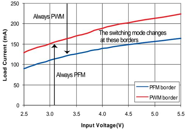
Figure 17. 1.233  $V_{OUT}$  PFM / PWM Boundaries
