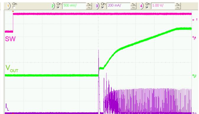
**Figure 38. Soft-Start,  $R_{LOAD} = 50\ \Omega$ ,  $20\ \mu\text{s}/\text{div}$ .**
