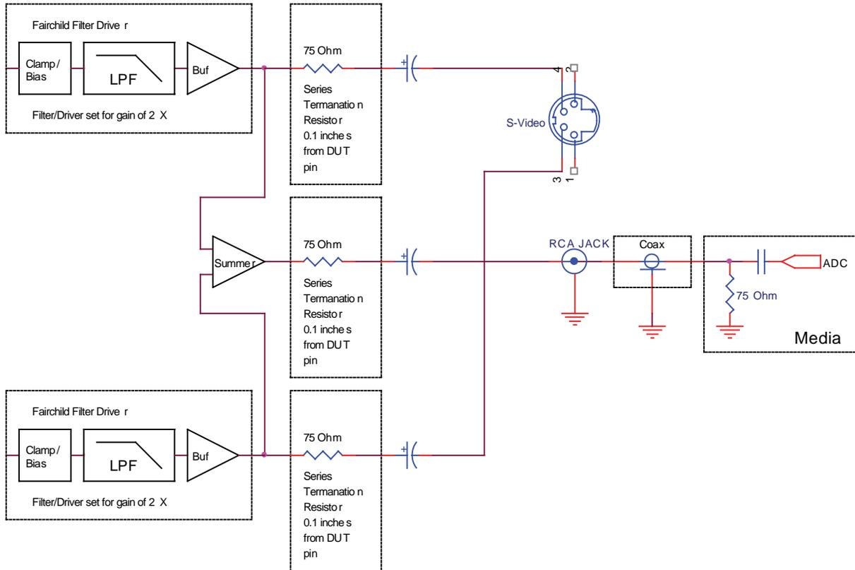
**Figure 5. Schematic Representation of a Video Filter / Driver**
