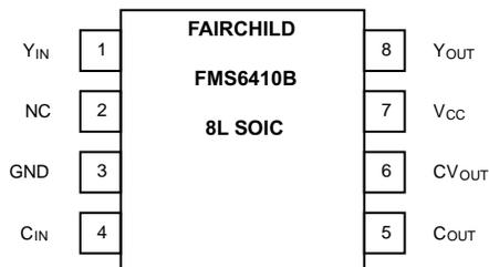
Figure 2. Pin Configuration
