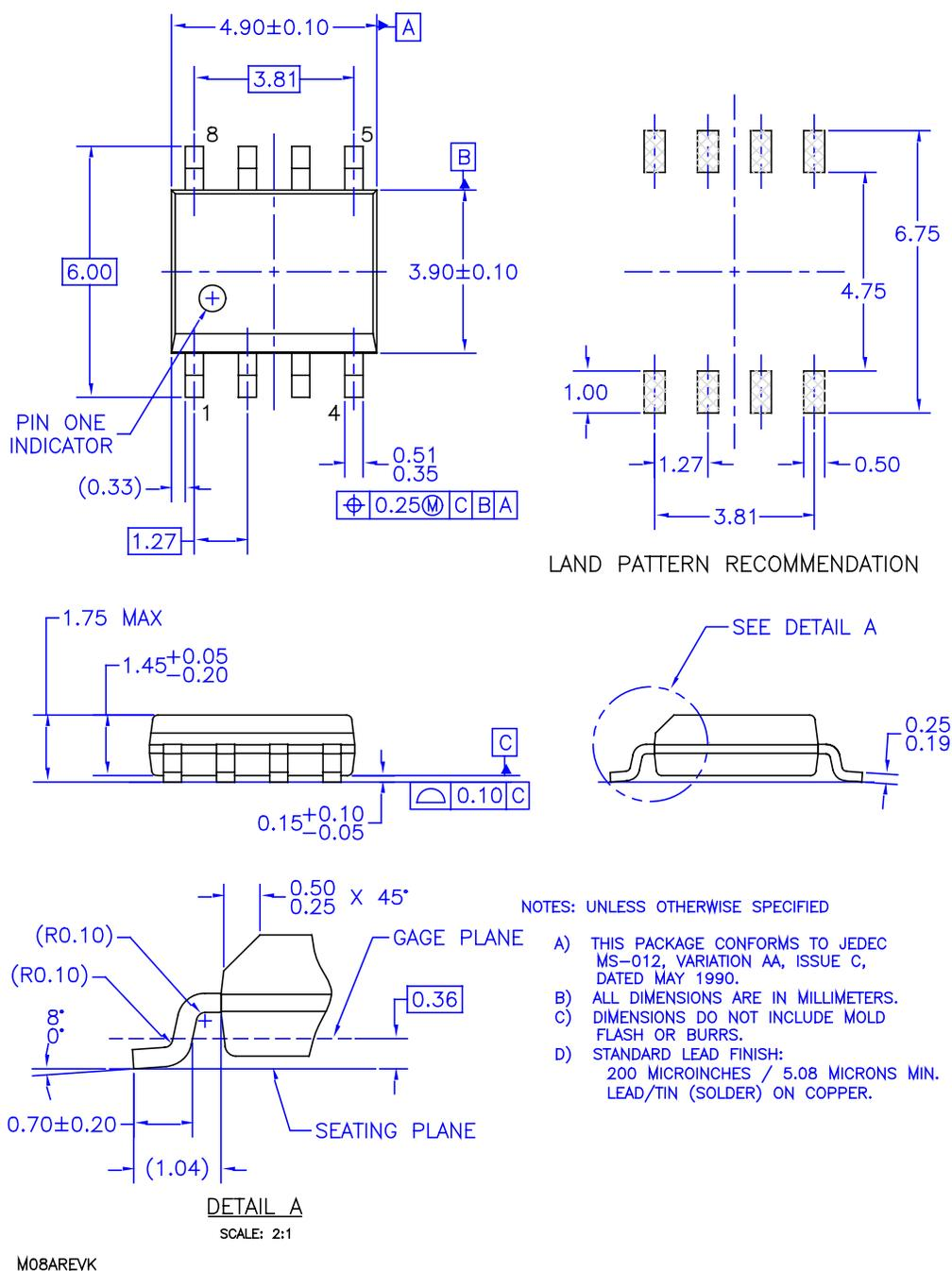
Figure 6. 8-Lead Small Outline Integrated Circuit (SOIC) Package
