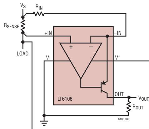
Figure 5. LT6106 Supply Current Monitored with the Load
