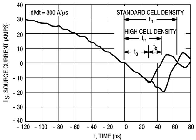
**Figure 11. Reverse Recovery Time ( $t_{rr}$ )**
