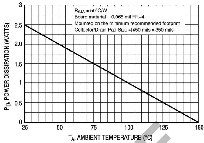
Figure 15. D<sup>2</sup>PAK Power Derating Curve
