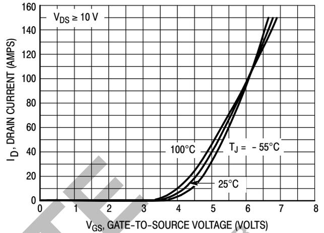
Figure 2. Transfer Characteristics
