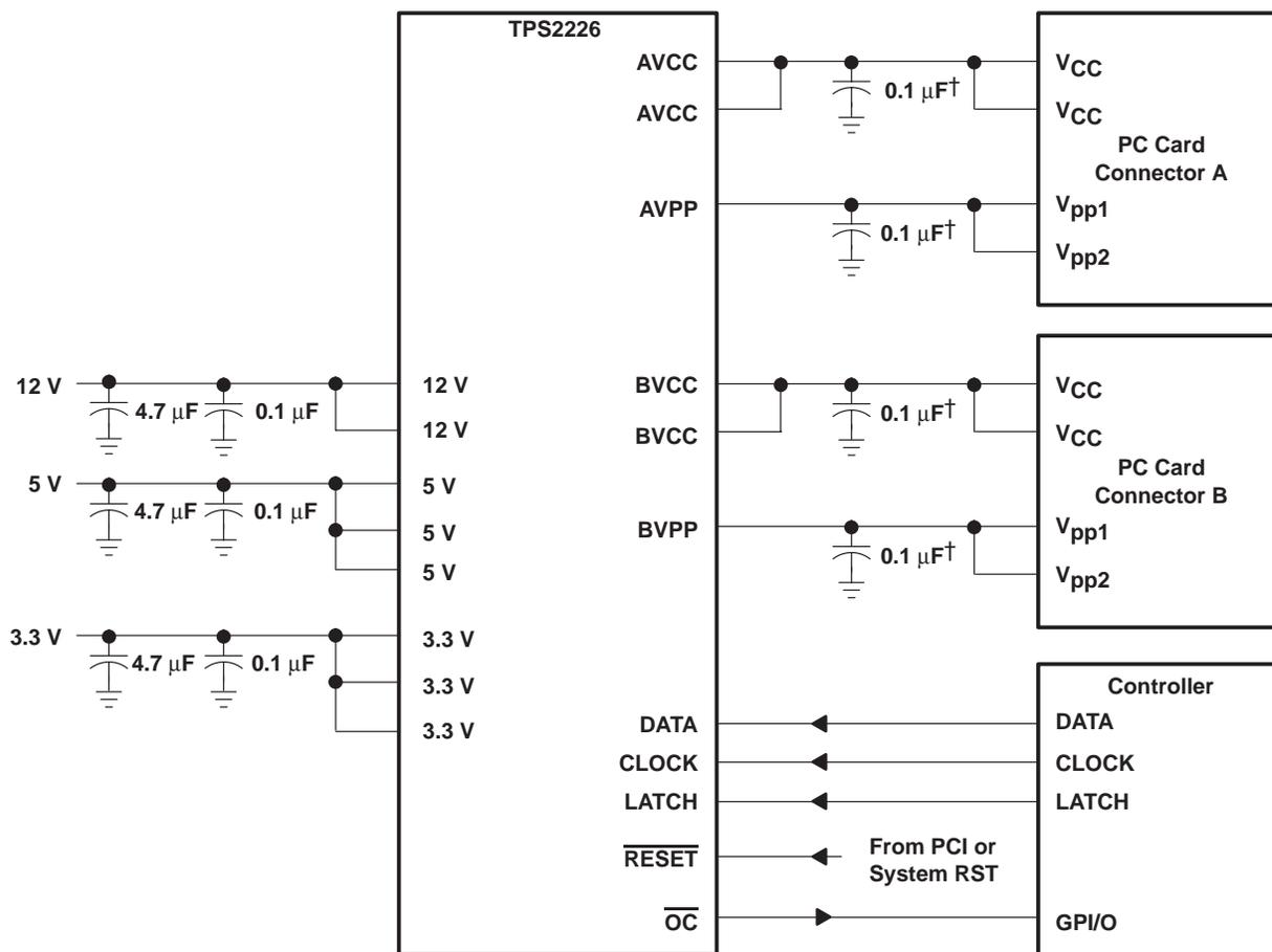
† Maximum recommended output capacitance for xVCC is 220  $\mu$ F including card capacitance, and for xVPP is 10  $\mu$ F, without  $\overline{OC}$  glitch when switches are powered on.
