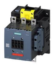
Power contactor, AC-3 115 A, 55 kW / 400 V Coil AC 50/60 Hz and DC 96-127 V x (0.8-1.1) F-SPS input 24 V DC 3-pole size S6 Auxiliary contacts 2 NO + 2 NC permanently mounted Main circuit: Busbar Control and auxiliary circuit: Screw terminal
