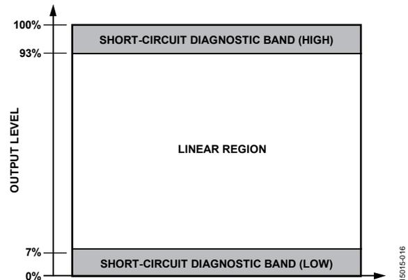
Figure 16. Output Span Classification During Short-Circuit Diagnostic Condition
