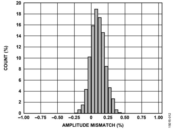
Figure 12.  $V_{SINx}$  to  $V_{COSx}$  Amplitude Mismatch Per Channel
