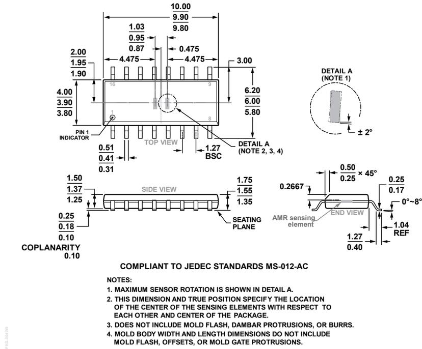
Figure 17. 16-Lead Standard Small Outline Package [SOIC\_N]
