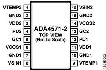
Figure 2. Pin Configuration
