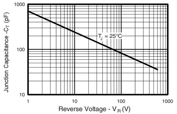
Fig. 3 - Typical Junction Capacitance vs. Reverse Voltage
