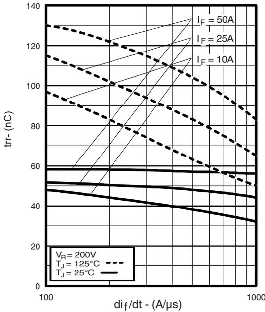
Fig. 5 - Typical Reverse Recovery Time vs.  $di_f/dt$
