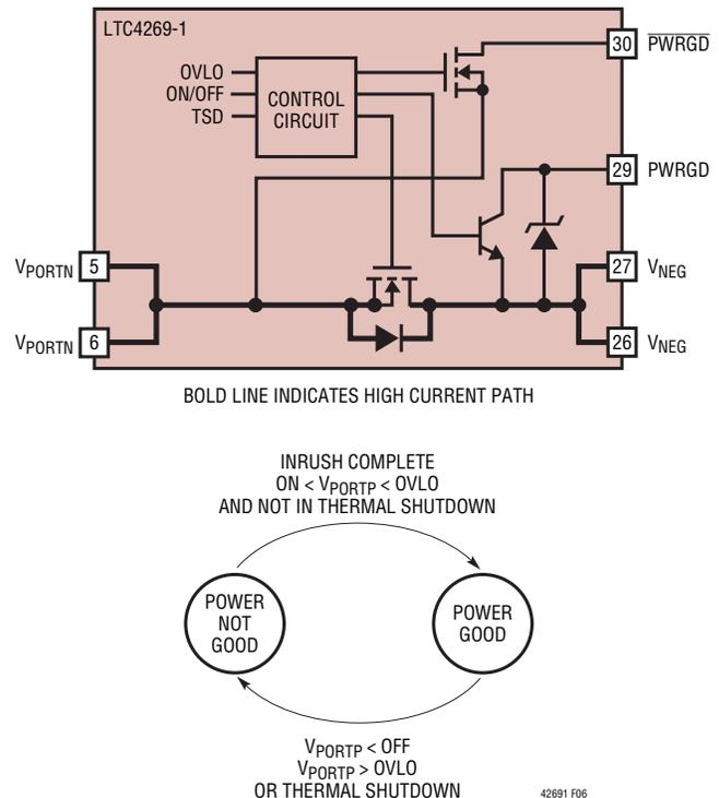
Figure 6. LTC4269-1 Power Good Functional and State Diagram
