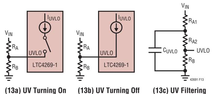
Figure 13. UVLO Pin Function and Recommended Filtering
