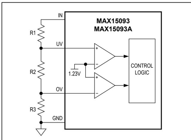
Figure 1. Undervoltage/Overvoltage-Threshold Setting
