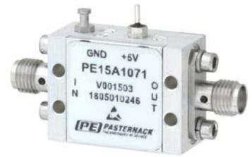
1.9 dB NF Low Noise Amplifier, Operating from 6 GHz to 18 GHz with 26 dB Gain, 13 dBm Psat and SMA
