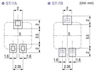
Note) The zero point is the center of mounting.
