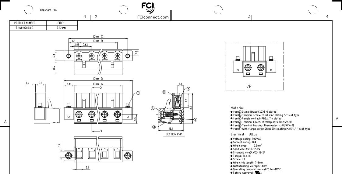
N = Number of poles Dim A=(N-1)X7.62+5.62Dim B=(N-1)x7.62Dim C=(N-1)x7.62+12.2Dim  $D=(N-1)\times7.62+18.0$
