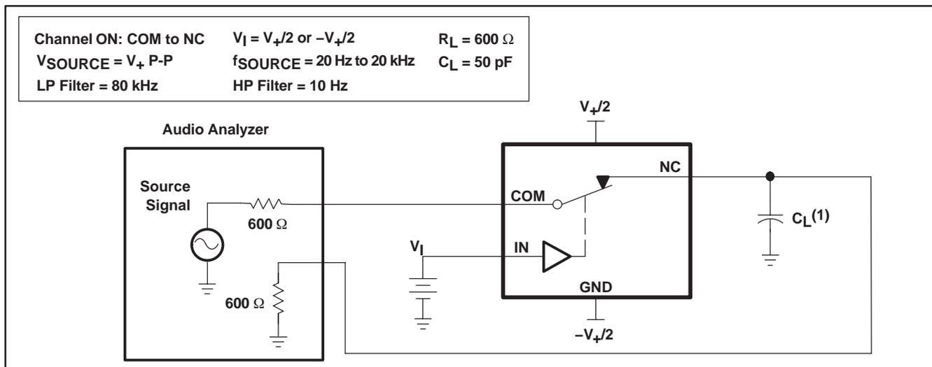
(1)  $C_L$  includes probe and jig capacitance.
