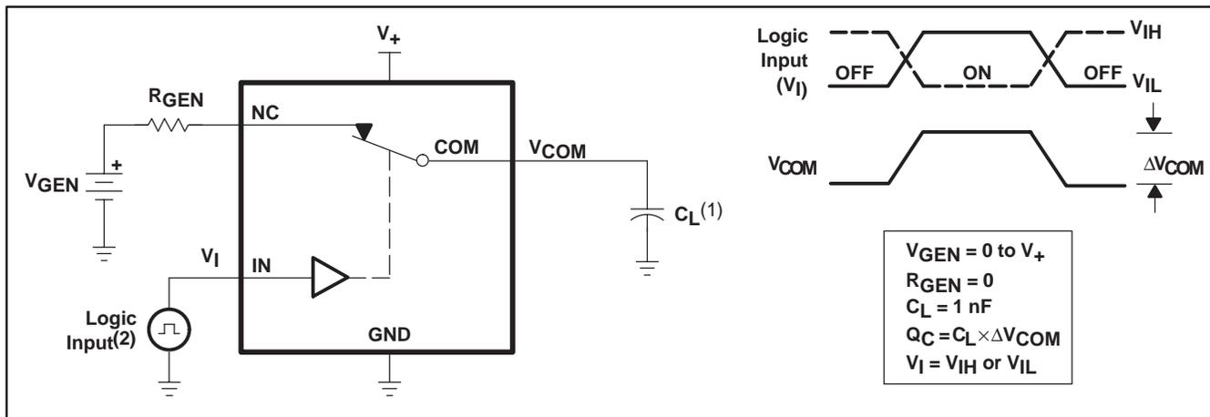
(1)  $C_L$  includes probe and jig capacitance.
