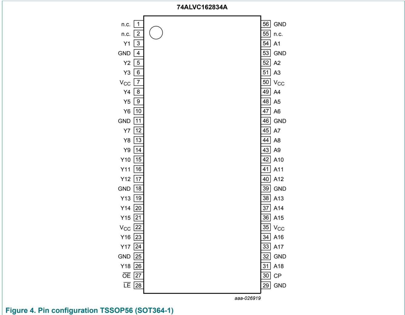
Figure 4. Pin configuration TSSOP56 (SOT364-1)
