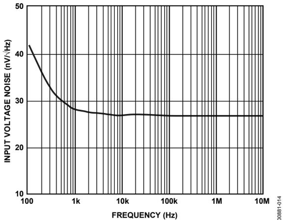
Figure 14. Noise Spectral Density
