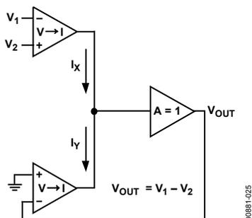
Figure 25. AD830 as a Difference Amplifier
