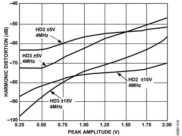
Figure 16. Harmonic Distortion vs. Peak Amplitude, Frequency = 4 MHz
