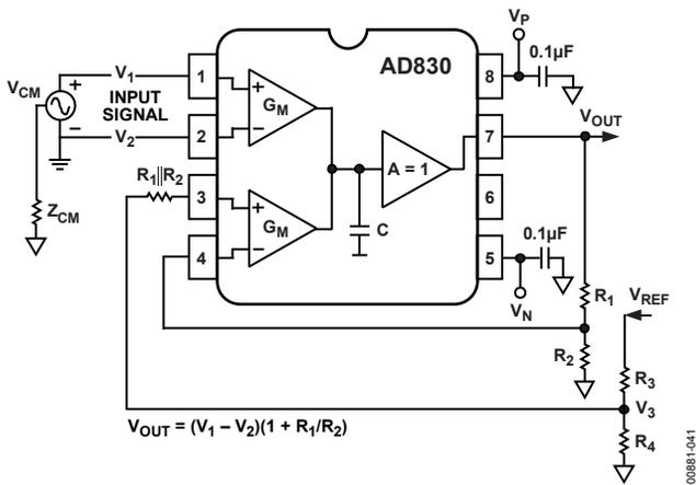
Figure 41. Offsetting the Output with Differential Gain > 1
