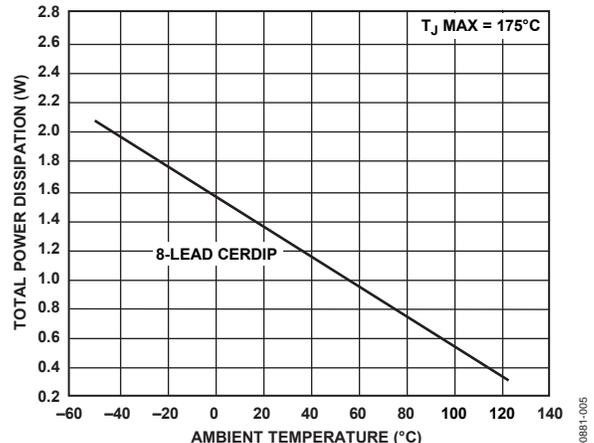
Figure 5. Maximum Power Dissipation vs. Temperature, CERDIP Package
