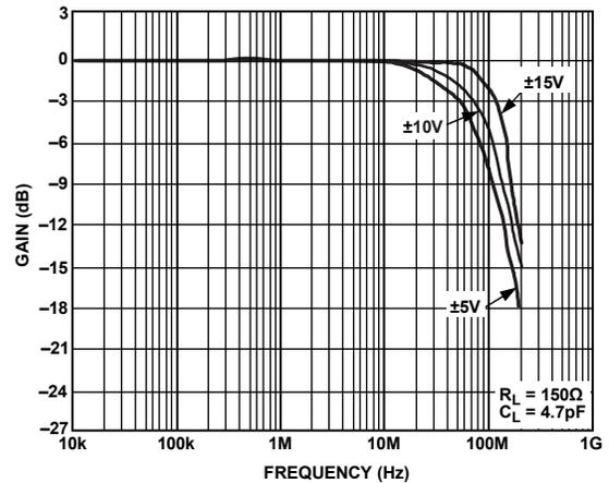
Figure 10. Closed-Loop Gain vs. Frequency G = +1
