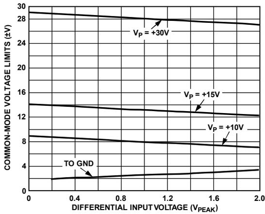
Figure 36. Input Common-Mode Range for Single Supply
