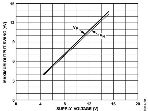
Figure 31. Maximum Output Swing vs. Supply
