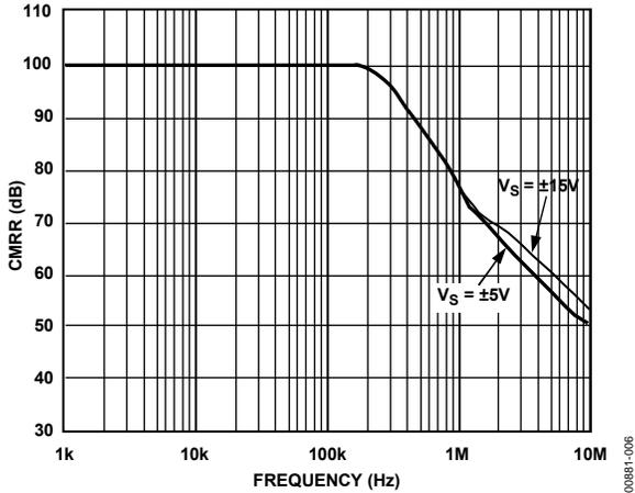
Figure 6. Common-Mode Rejection Ratio vs. Frequency
