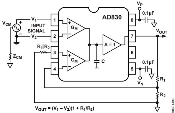
Figure 40. Gain of G Differential Amplifier,  $G > 1$
