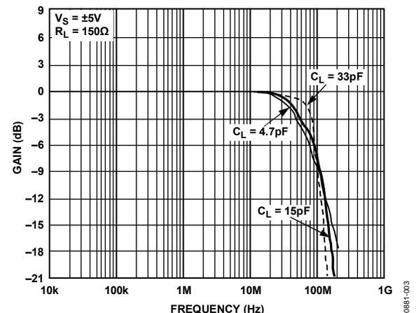
Figure 3. Closed-Loop Gain vs. Frequency, Gain = +1
