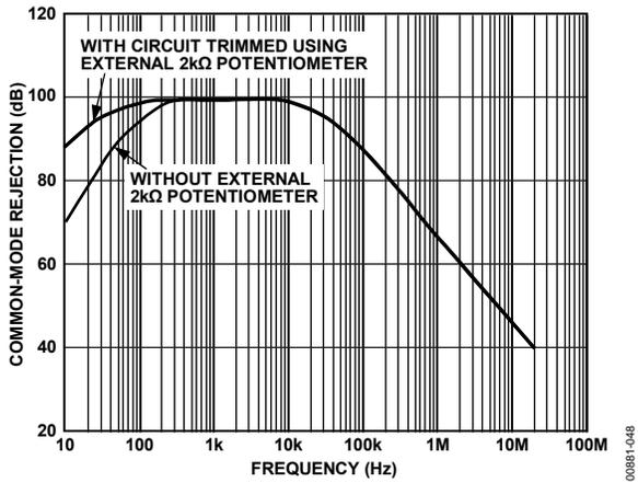
Figure 48. Common-Mode Rejection vs. Frequency for Line Receiver
