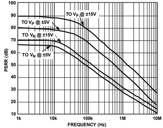
Figure 9. Power Supply Rejection Ratio vs. Frequency
