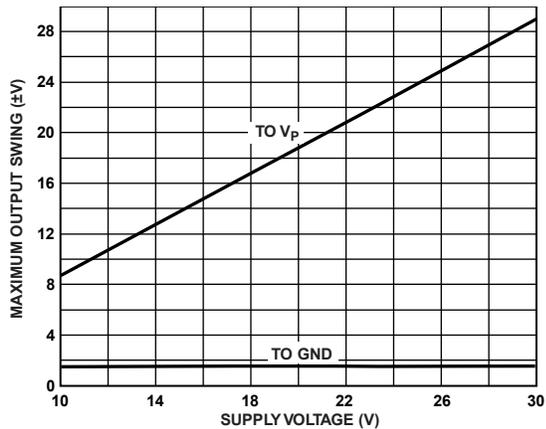
Figure 37. Output Swing Limit for Single Supply
