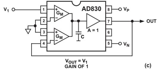
Figure 21. Connection Diagrams
