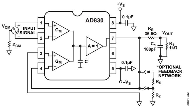
Figure 32. Circuit for Driving Large Capacitive Loads
