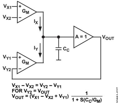
Figure 27. Closed-Loop Connection
