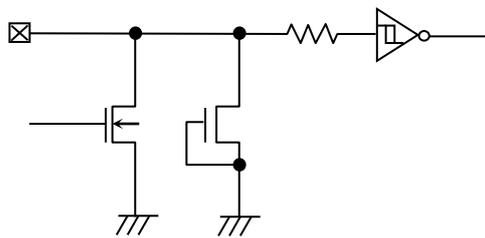
Figure 50. Input / Output Pin Circuit Diagram
