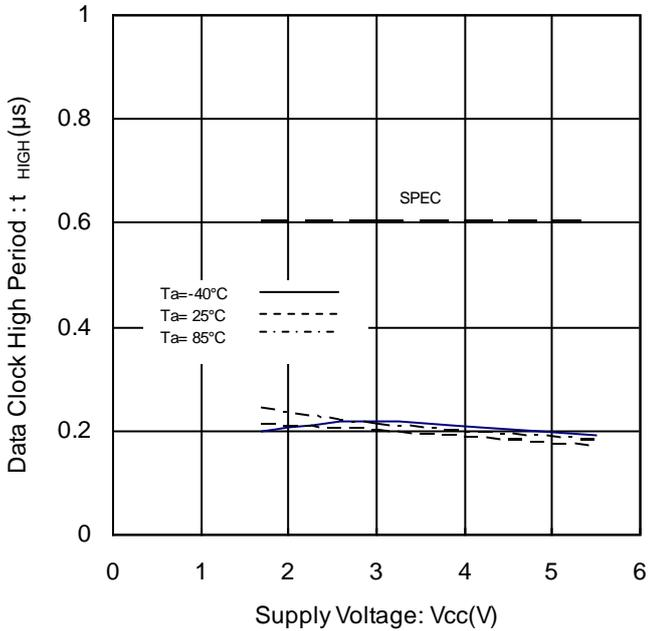
Figure 14. Data Clock High Period vs Supply Voltage
