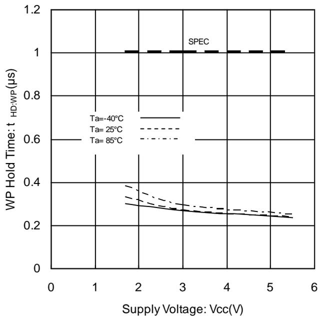
Figure 31. WP Hold Time vs Supply Voltage
