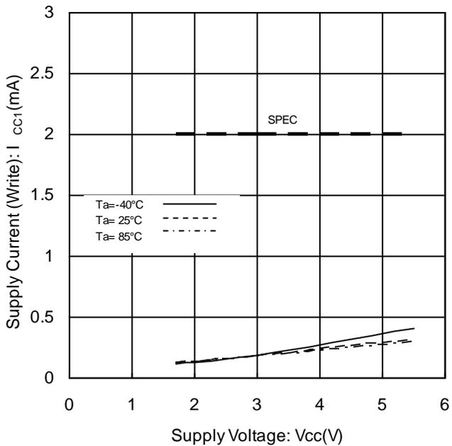
Figure 10. Supply Current (Write) vs Supply Voltage (f<sub>SCL</sub>=400kHz)
