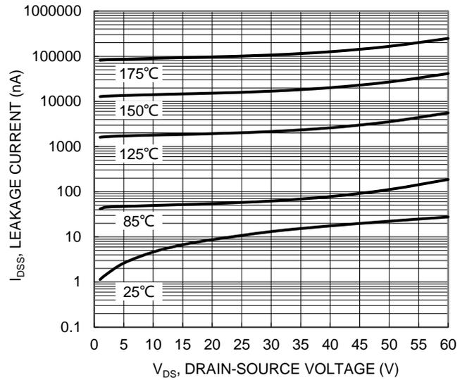
Figure 10. Typical Drain-Source Leakage Current vs. Voltage
