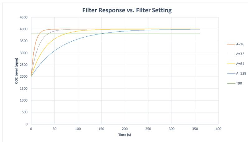
The graph above shows the effect of the filter on response times. Increasing the filter setting increases the measurement output response time. T<sub>90</sub> is the time to 90% of reading. The ExplorIR®-W takes 2 readings per second.
