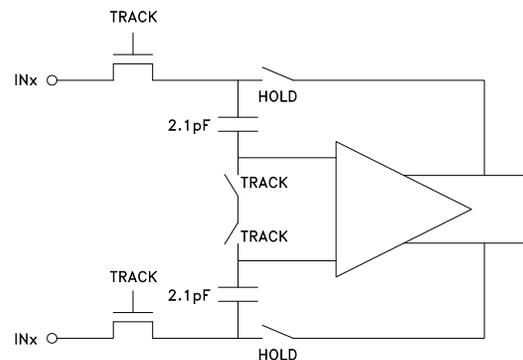
Figure 4: Input configuration
