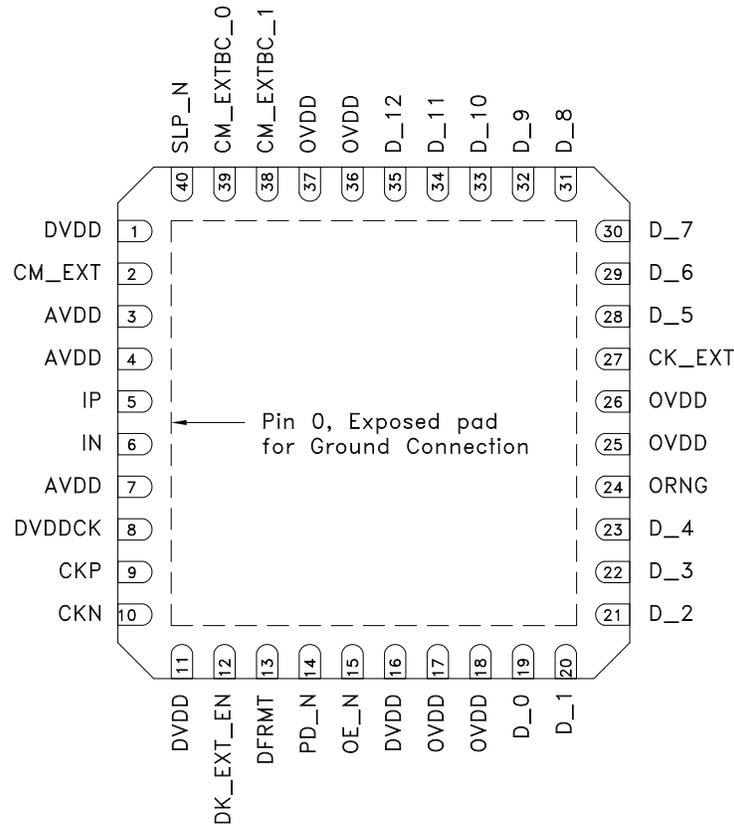
Figure 3: Package Drawing, QFN 40-pin
