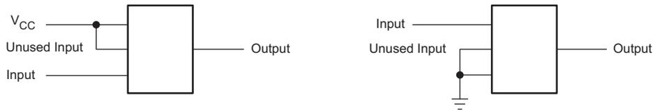
Figure 7. Layout Diagram
